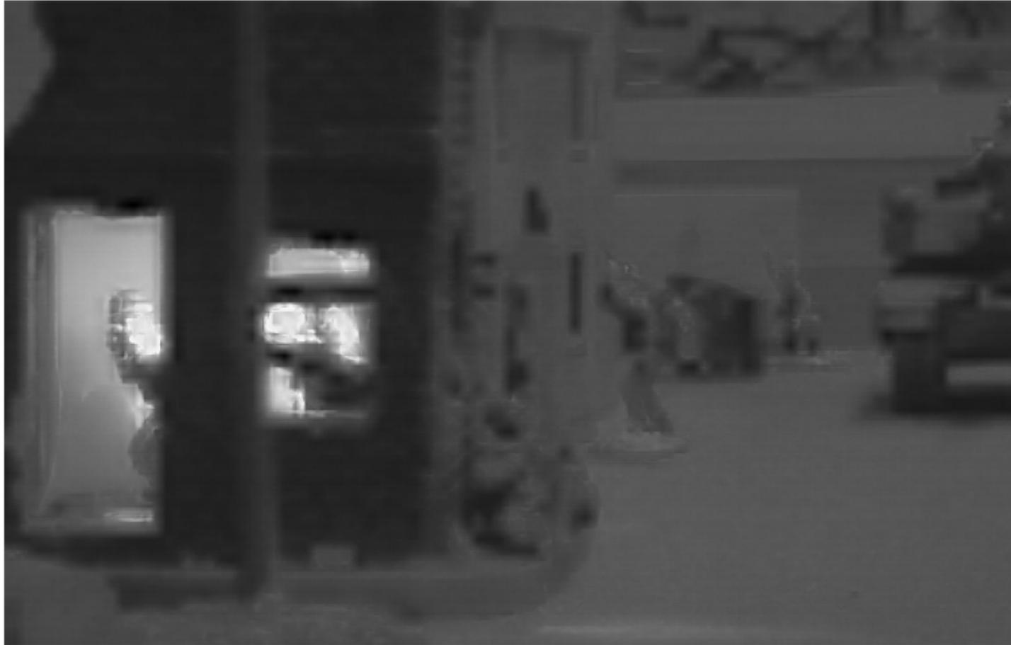
Figure 34: Oversaturated output of DWT-based framework from modified  $\alpha$  values in DRC
