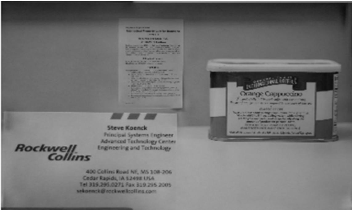
Figure 20: Area-based multi-focal fusion algorithm minimizes artifacts but has lost detail
